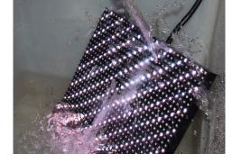
The tiles are rated at IP67, meaning they can be fully submerged in water.
